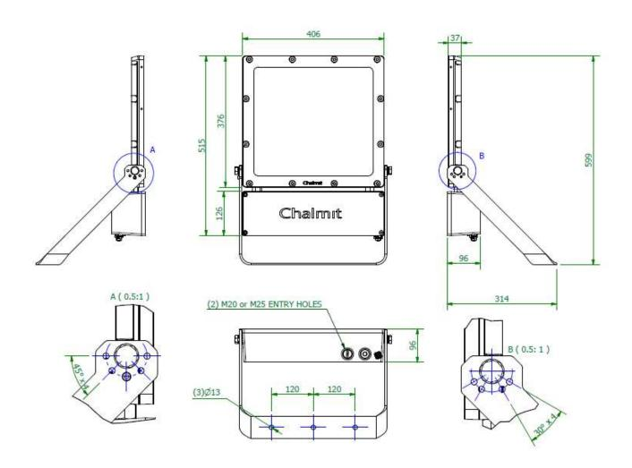
THE EVOLUTION X STIRRUP BRACKET HAS PRE-DEFINED FIXING ANGLES ALLOWING YOU TO AIM THE FLOODLIGHT AT INCREMENTS OF 30° OR 45° PLEASE REFER TO DIAGRAM ABOVE
